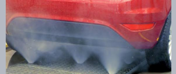
Possible choice: static underchassis wash 10 bar [145 PSI] 90 L/min [23.8 gpm], oscillating 15 bar [217 PSI] 120 L/min [31.7 gpm], or by sector 15 bar [217 PSI] 120 L/min [31.7 gpm].
